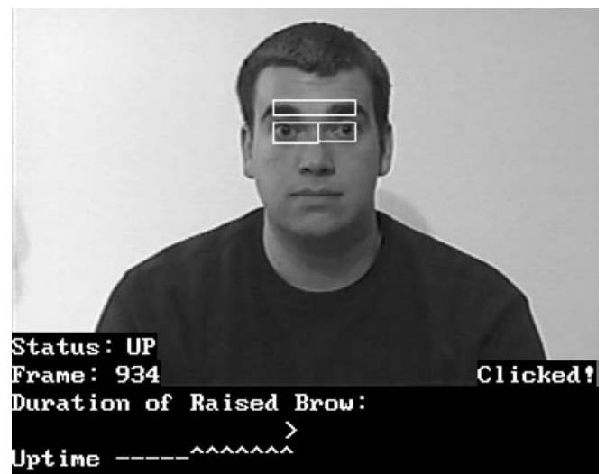
Fig. 8. A user of EYEBROWCLICKER immediately after issuing a “click” as a selection command. The bar on the bottom displays the duration of the current eyebrow-raising action
