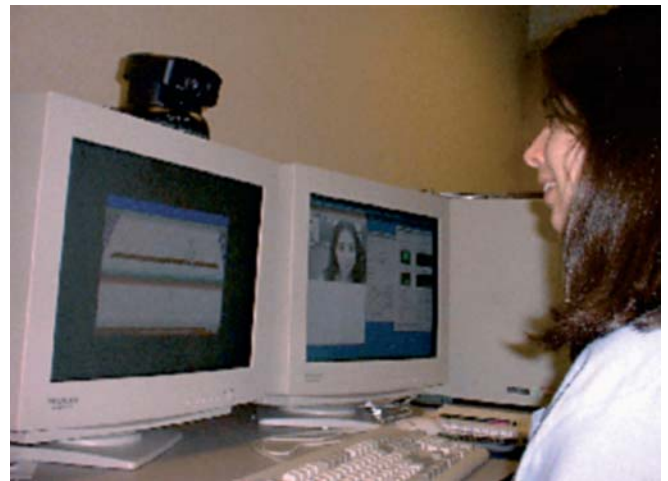
Fig. 12. BLINKLINK in use: the video camera is placed on top of the left monitor, which displays the application software. The right computer monitor (not required) is used to check the status of the system. A user plays an arcade game based on scanning software where the objective is to throw a baseball at plates on a shelf. A long blink causes a ball to be thrown. The user must time the blink so that it coincides with the highlighting of a plate
