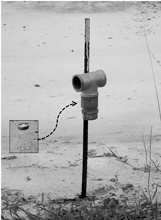
Fig. 1 Scent dispenser used to emit 3-mercapto-3-methylbutanol (3-M-3-MB) or a mixture of volatile acids and piperidone (VA+P). A 10-ml septum-capped vial charged with scent ( inset ) or a 22-ml open-topped vial (not shown) is held within the stem of the T-shaped head , which is made from 25-mm pipe connectors
