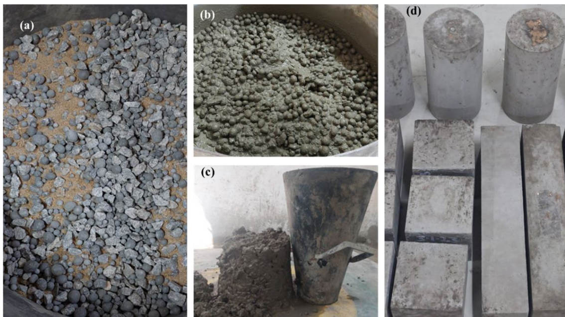
Fig. 9 Concrete production a Dry mixing of raw materials, b Fresh concrete, c Slump measurement, d Concrete samples after demoulding
