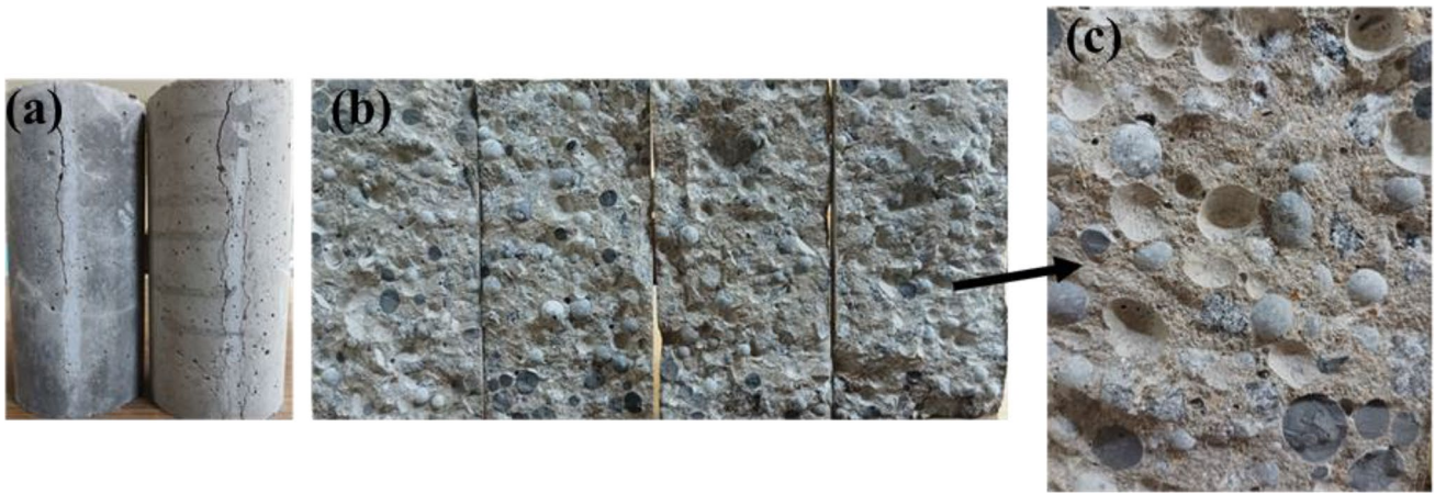
Fig. 15 Failure of specimens a Failure pattern, b, c broken surfaces
