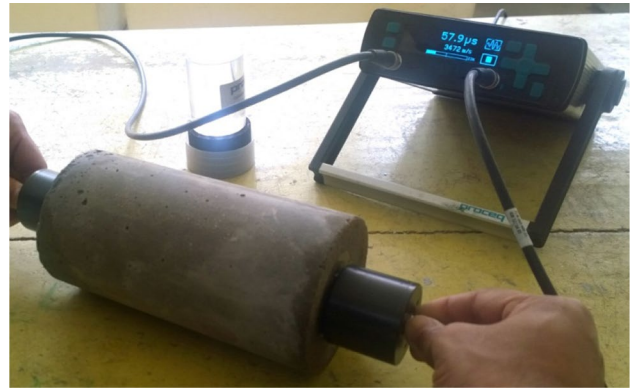
Fig. 3 Measurement of UPV
