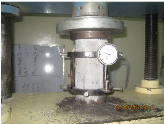
Fig. 2 Measurement of deformation under compression load
