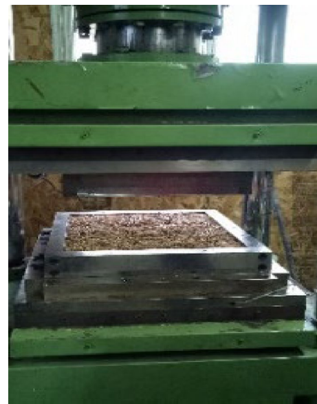
Fig. 2 Hot pressure for particleboard manufacturing. The gauge ram of the hot pressure: 15 cm; the temperature of the top and bottom plates < 200 °C; the pressure is 100 kgf/cm 3
