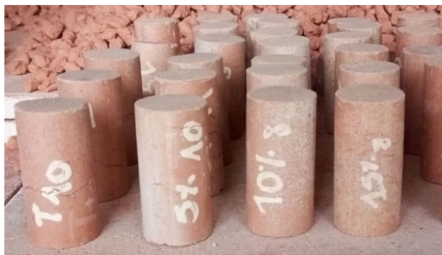
Fig. 8 Visible cracks on control bricks (T10) and (5% 10) fired at 1000 °C and white film on the surface of 5%, 10% and 15% bricks
