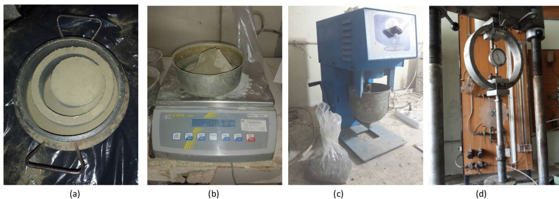
Fig. 2 Sludge grinding (a), preparation of mixtures (b), mixing (c) and moulding (d)
