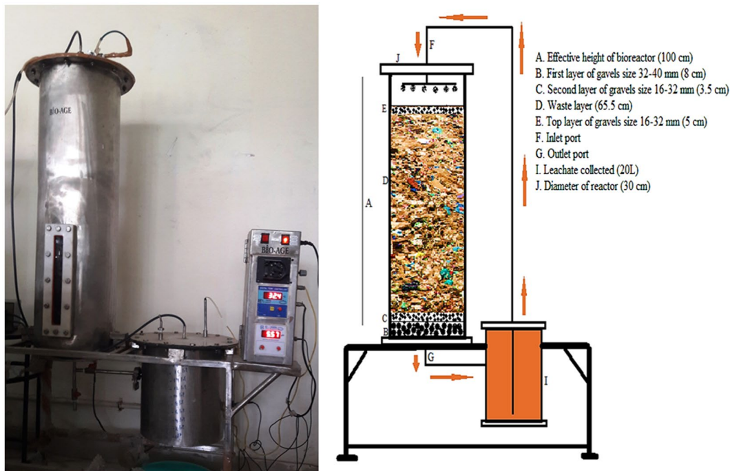
Fig. 1 Lab-scale leachate recirculation bioreactor
