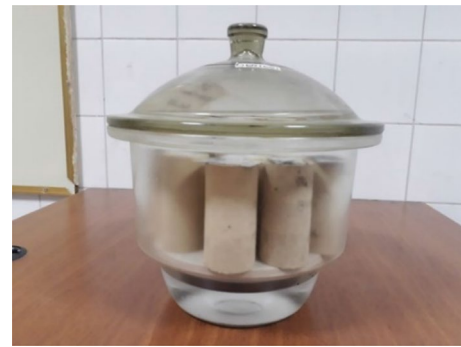
Fig. 5 Specimens in desiccator cabinet
