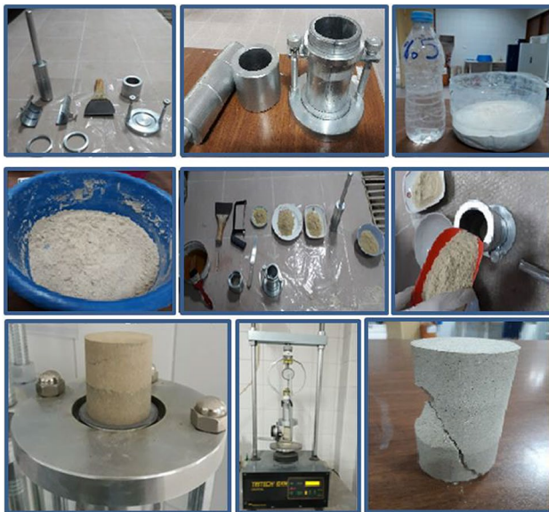
Fig. 4 The preparation of soil specimens and UCS tests
