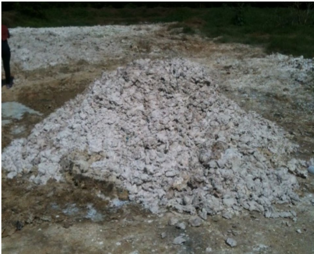
Fig. 1 Sludge waste from manufacturing process of the concentrated natural rubber latex in landfill
