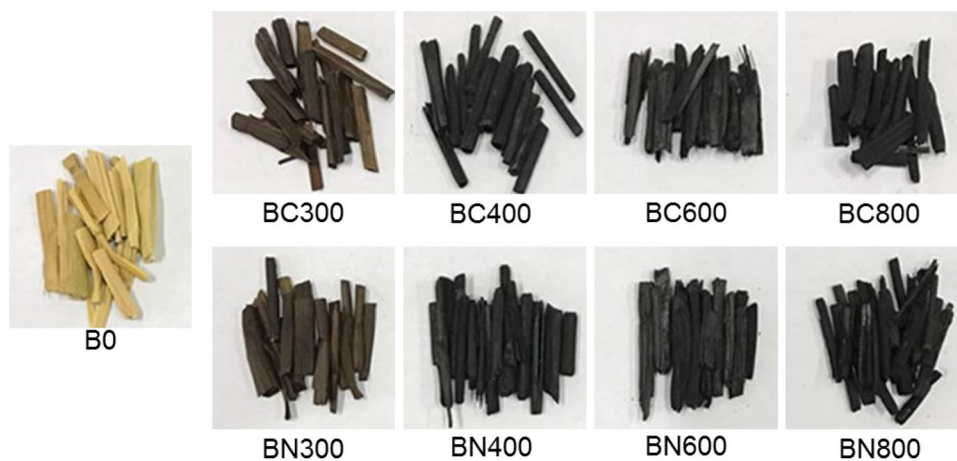
Fig. 1 Straw and the biochars prepared under different conditions
