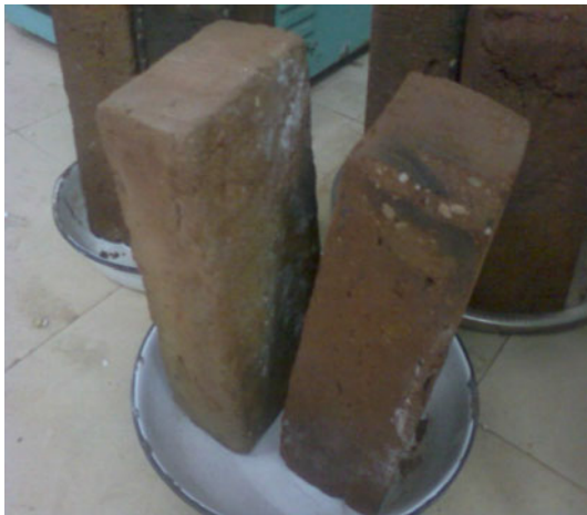
Fig. 7 Liability of efflorescence on the brick
