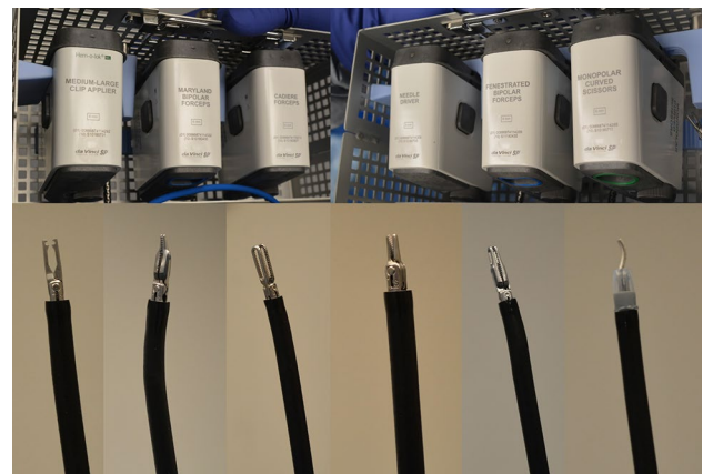
Fig. 4 Single-port instrument tips and bases. From left to right, medium-large clip applier, Maryland bipolar forceps, Cadiee forceps, needle driver, fenestrated bipolar forceps, and monopolar-curved scissors
