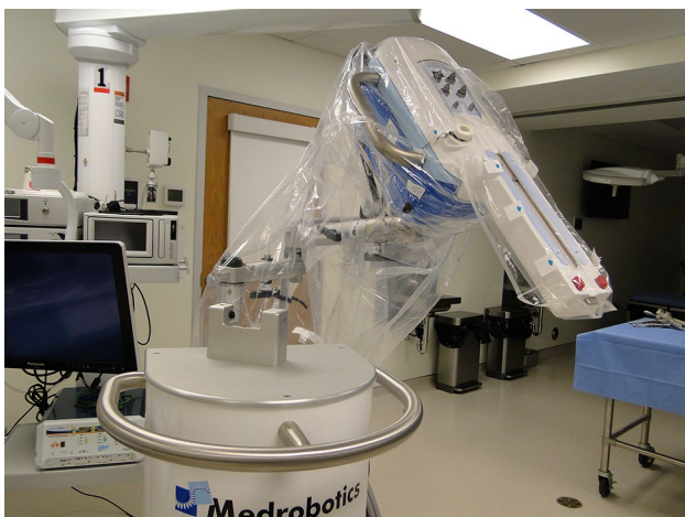
Fig. 2 Flex® Robotic Base (draped) is shown. This accommodates the Flex® Robotic Colorectal Drive, which has recently received Federal Drug Administration 510(k) clearance in the USA
