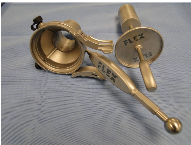
Fig. 5 The single-use Flex ® Robot Colorectal Drive is mated to this specially designed and reusable access channel. Thus, some aspects of the apparatus are disposable, while others are reusable
