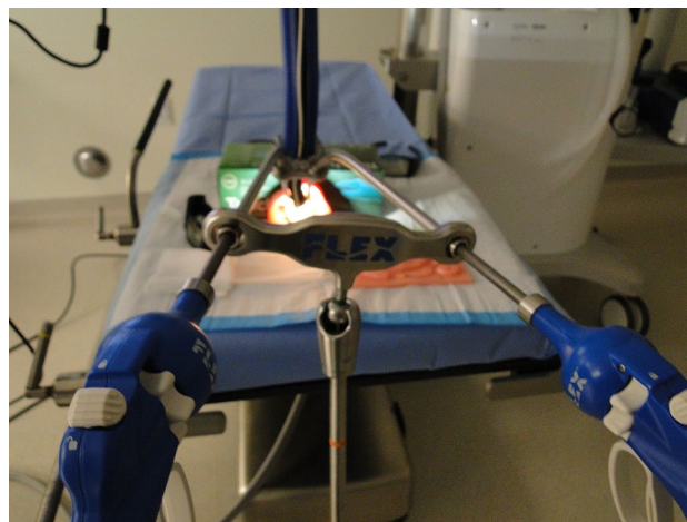
Fig. 4 Flex Robot System with Colorectal Drive is docked transanally. In this configuration, the Flex Robot is at the 12 o'clock position, and an 8 mm AirSeal trocar is positioned at 6 o'clock and is connected to a high-flow insufflator for stable pneumatics. At the 3 and 9 o'clock position are metal tubes through which the flexible instruments are delivered (within the access channel these tubes become flexible). The entire system is secured to the operating table rail by mounts so as to provide platform stability
