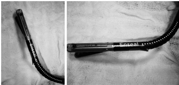
Fig. 2 ENSEAL ® device breaks—repeated articulation and disarticulation of the device can result in a break where part of the shaft where current flows arches out
