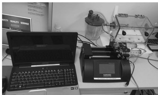
Fig. 1 Burst pressure apparatus—a setup of the device used to measure the burst pressure of the seals. Vessels were sealed, sutured to the device and then filled with a constant infusion of saline
