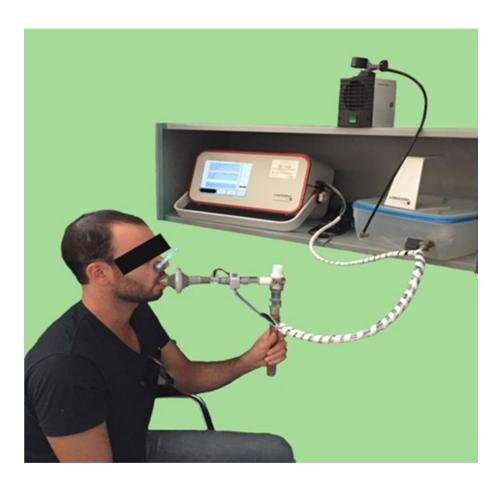
compact  $(92 \times 190 \times 255 \text{ mm})$  and lightweight (2.3 kg) portable olfactory system, consisting of a gas sampling unit and a sensor array. Using a pattern recognition software (Win Muster v. 1.6.2), the PEN3 allows visualization and analysis of the data and works using filtered ambient air during the cleaning step or dilute gas during sampling with a maximum flow rate of 600 ml/min.
