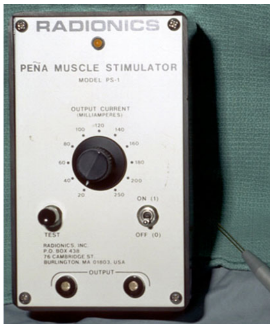
Fig. 1 Peña muscle stimulator used to identify the levator ani, puborectalis and external sphincter fibers during closure
