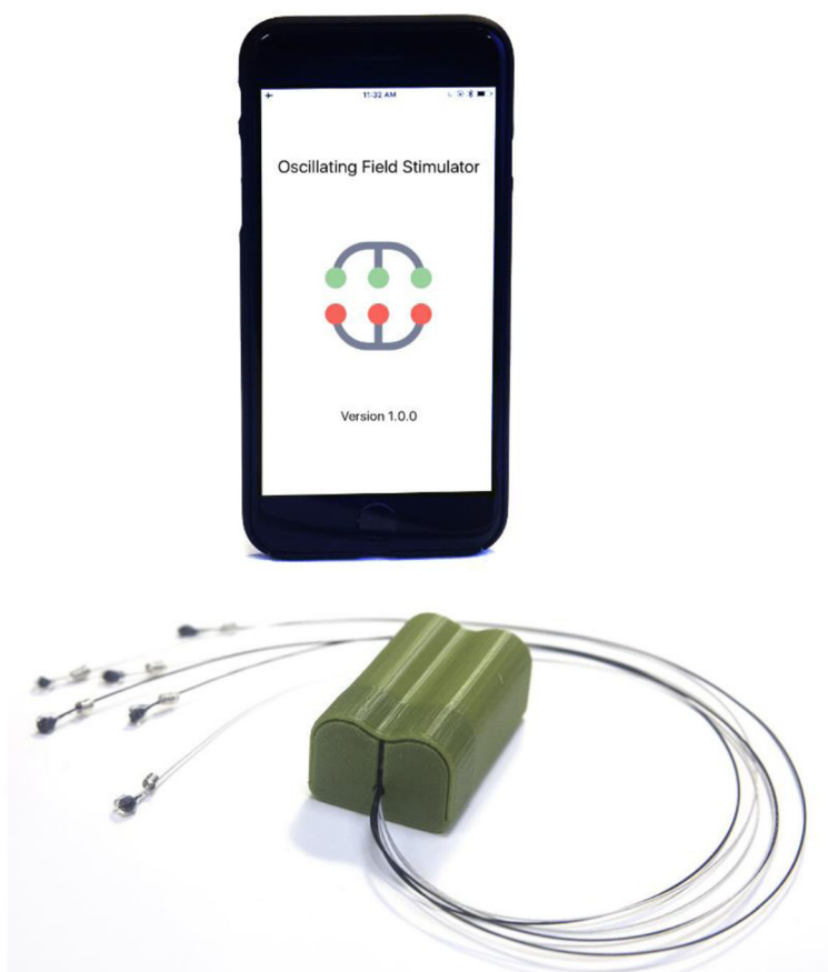
Fig. 3 Left: Image of a prototype OFS implant with a 3-D printed polymer casing. The size of the implant is comparable to that of a camera battery. The OFS communicates with the Apple-based iOS devices
