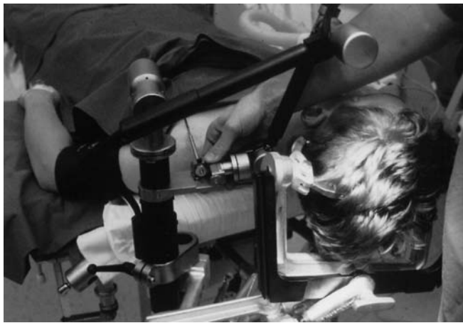
Fig. 4 Intraoperative calibration of the operating arm system (OAS), an arm-based navigation device
