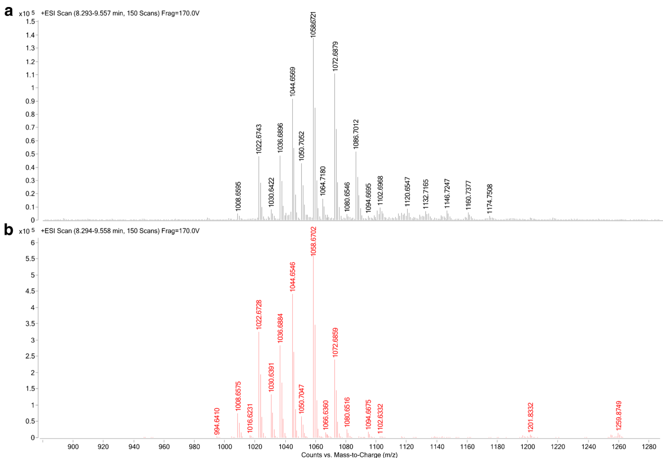
Fig. 5 LCMS analysis. Mass spectrometry profile for the biosurfactant produced by isolate AM13. X-axis represents the m/z ratio; Y-axis represents the abundance (count) of each fragment. a Mass spectrum of the extract of isolate AM13. b Mass spectrum of the standard surfactin used
