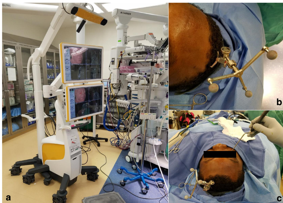
Fig. 13 CT-guided, computer-aided orbital reconstruction in a patient with orbital fracture. a The infrared camera and receiver mount with monitors for CT-guided navigation. A reference arc with reflective markers attached to a rigidly fixed headset is shown ( b ). Both the headset and a surgical instrument fitted with a reflective sphere are illustrated in c
