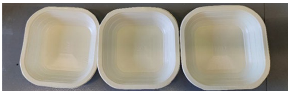
Fig. 16 Thermoformed items with B-TPS1 compound: as-is (left); after being tested at 65 °C (middle); after being tested at 100 °C (right).
