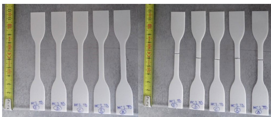
Fig. 12 B-TPS1 film samples in transversal direction before and after fracture.
