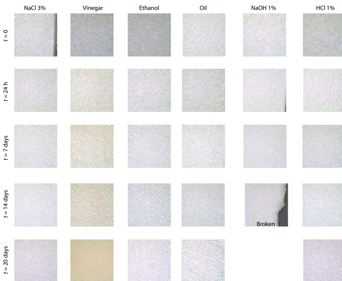
Fig. 15 Chemical inertia carried out on B-TPS1 films by cast extrusion.
