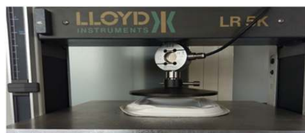
Fig. 18 Compression tests performed on the thermoformed items.
