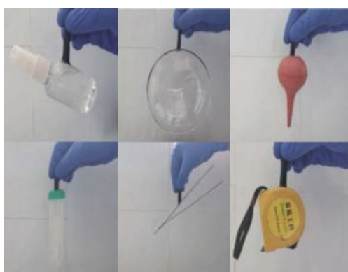
Fig. 7 Photographs of conductive hydrogel adhered to plastic, glass, rubber, and metal.
