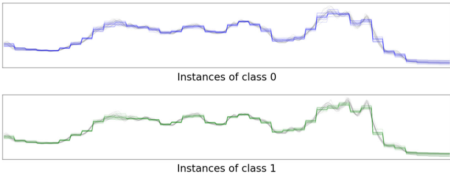
Fig. 2 Illustration of the PAA version of time series instances superimposed on their real-valued counterparts. The 286 time points long time series have been reduced to 40 time points based on a dimensionality reduction factor w = 7 . The PAA versions have been stretched (along the x-axis) to emphasize the retention of the overall shape of time series instances (color figure online)
