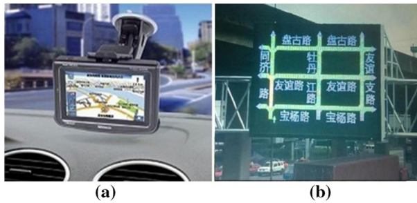
Fig. 4 Examples of in-vehicle and out-of-vehicle guidance systems ((a) shows an example of in-vehicle navigator and in (b), the green line means low traffic volume, the yellow line means moderate traffic volumes, and red means traffic congestion) (color figure online)
