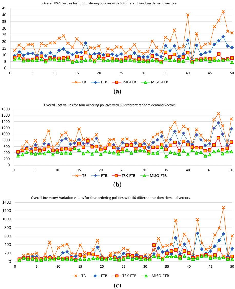
Fig. 14 a–c Scatter plots of overall BWE, cost and inventory variation values for TB, FTB, TSK-FTB and MISO-FTB token-ordering policies with fifty different random demand vectors. a Overall BWE values for TB, FTB and proposed fuzzy ordering policies with 50 different random demand vectors. b Overall cost values for TB, FTB and proposed fuzzy ordering policies with 50 different random demand vectors. c Overall inventory variation values TB, FTB and proposed fuzzy ordering policies with 50 different random demand vectors
