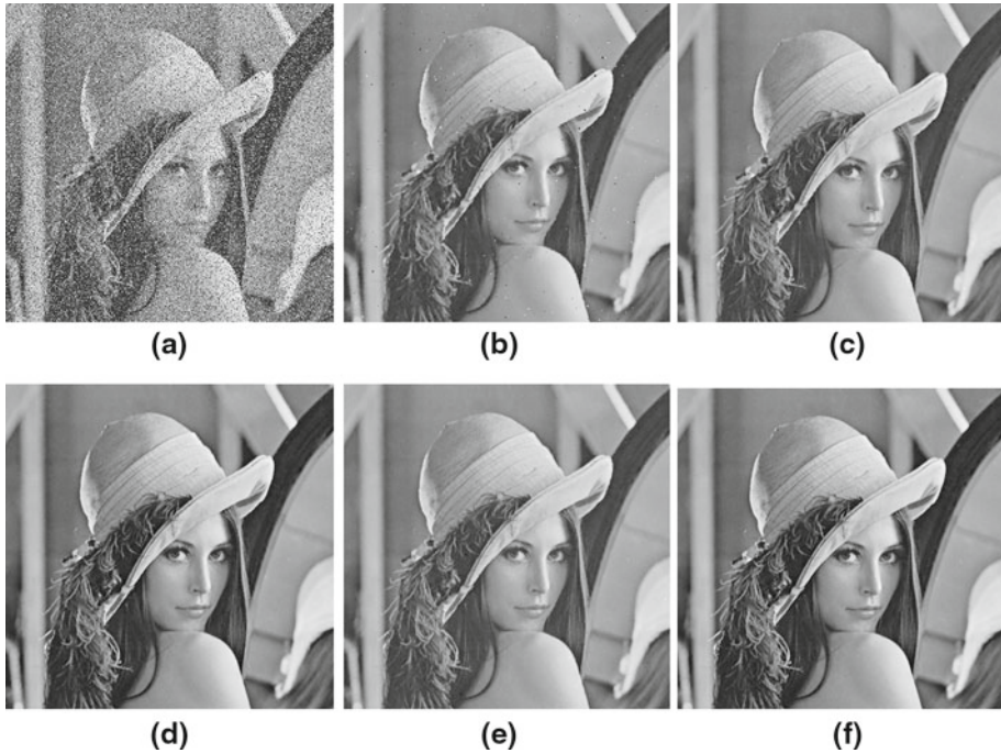
Fig. 10 Performance comparison of image restoration results obtained from the LENA image using different algorithms. a Image corrupted with 20% salt-and-pepper noise, b SMF (29.47 db), c PSMF (34.79 db), d DBA (37.33 db), e NIDF (34.04 db), and f proposed method (39.18 db)
