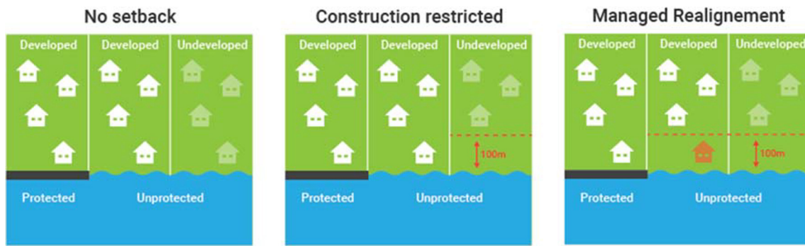
Fig. 3 Schematic presentation of the different setback approaches used in the study. White houses exist, while light green houses represent future construction, and red houses exist but are in the phase of depreciation and thus will disappear
