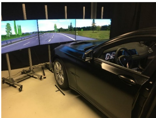
Fig. 1 Static driving simulator with mockup and three front channels used in the current study
