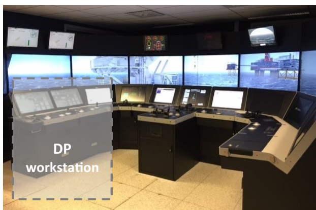
Fig. 1 Full-mission bridge simulator K-Sim® DP (copyright: Kongsberg Group)
