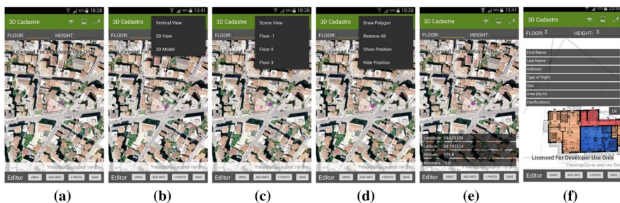
Fig. 6 Overview of the developed application supporting the proposed crowdsourcing procedure for initial registration of 3D cadastral data. a The mobile application's user interface b tools for adjusting the viewing mode of the scene c basemap selection tools d polygon drawing tools e representation of GPS coordinates (Show position tool) f representation of input information fields (ADD INFO)
