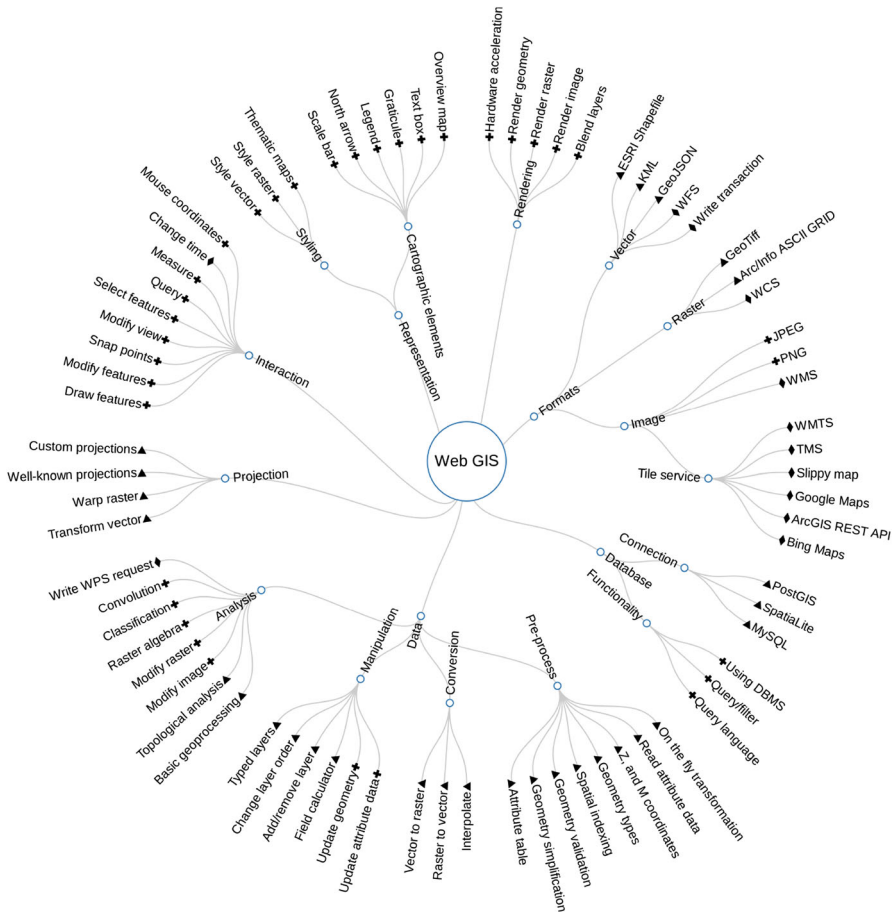
Fig. 1 Possible features of a basic Web GIS application grouped by functionality. Triangles, crosses, and diamonds denote GIS-specific features, non-GIS-specific features, and web mapping-specific features, respectively
