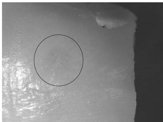
Fig. 5. Discoloration (circle) of the tooth specimen at 9 \text{ J/cm}^2 and a pulse duration of 350 \mu\text{s} (LP pulse). This tissue alteration in the region of the threshold energy density was not rated as ablation.
