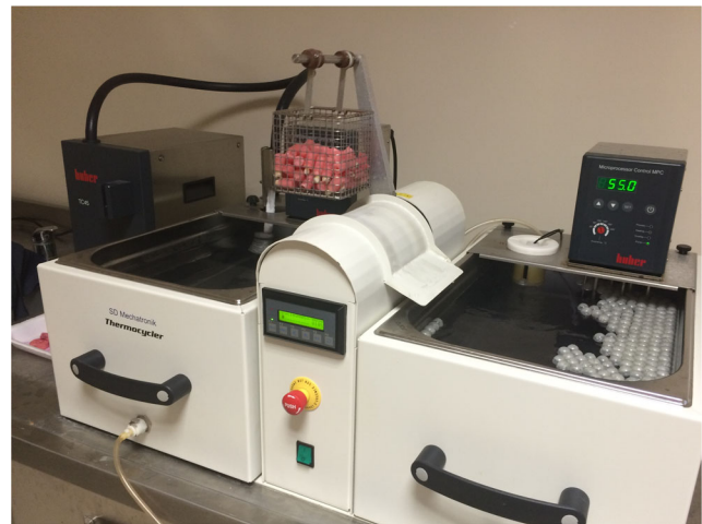
Fig. 1 The bonded specimens were stored in artificial saliva and incubated at 37 °C for 24 h, followed by a thermocycling process (5000 cycles, 5–55 °C)
