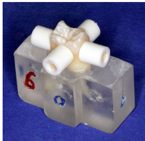
Fig. 3 Fixed composite rods in the Gütermann beads on the dentin surfaces a, b, c and d in the sample 6
