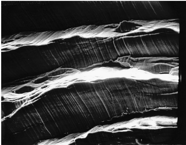
Fig. 14. The SEM Photograph of the rough side of Ti-6Al-4V chip cut under cryogenic machining conditions
