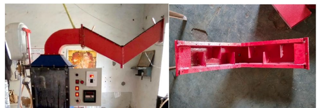
Fig. 11 Image of dehumidifier with baffle plates (Thanaiah et al. 2021) with permission from Elsevier
