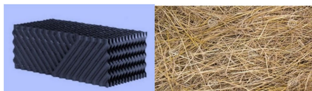
Fig. 7 Image of packing materials (polypropylene and paddy grass) (Thanaiah et al. 2021) with permission from Elsevier
