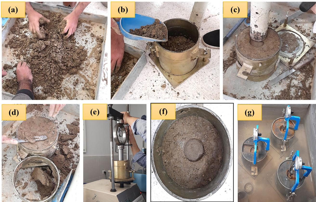
**Fig. 18** Stages of sample preparation for CBR testing **a** hand-mixing of soil and guar gum powder, **b** sample pouring in CBR mold for compaction, **c** layer-by-layer compaction of soil-GG mix in CBR mold by modified Proctor hammer, **d** trimming and leveling of the
