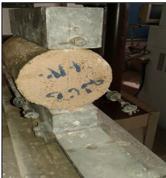
Fig. 6 Splitting tensile strength test
