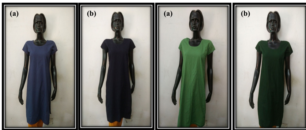
Fig. 10 Images of a conventional and b cationized cotton dyed garments
