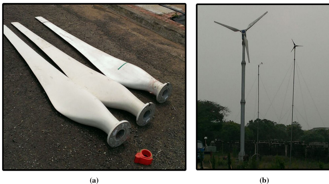
Fig. 7 a 10 kW turbine blade and b operational system located in Tainan, Taiwan
