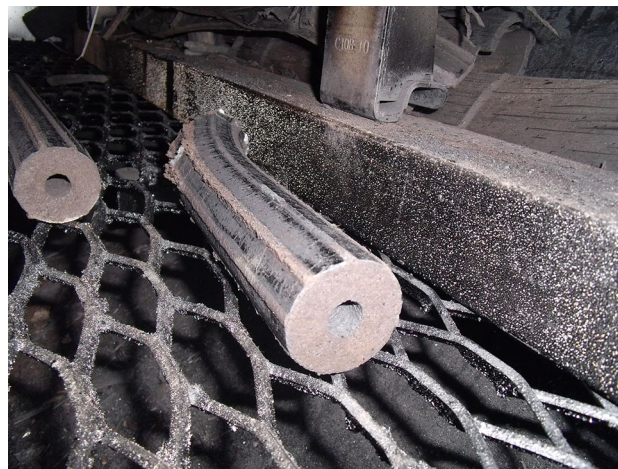
Fig. 3 The charcoal dust of a negligible price was mixed with conventional solid plant biofuels. This cheapened the cost, but increased the heating value and combustion temperature leading to improved hygienic indicators and better combustion characteristics in total
