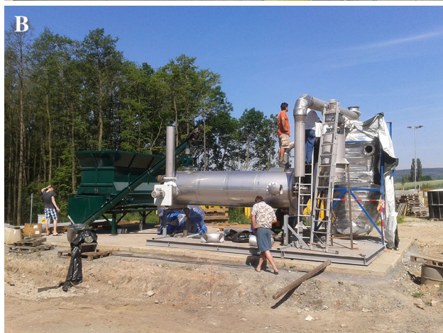
Fig. 2 The technology unit is first of its kind in a commercial size. The feeding mechanism is captured on the left ( green ). The outside wall of the pyrolysis reactor is located in the middle in a horizontal position. The heat exchanger (to utilize the waste flue gases) is located on the right. (Color figure online)
