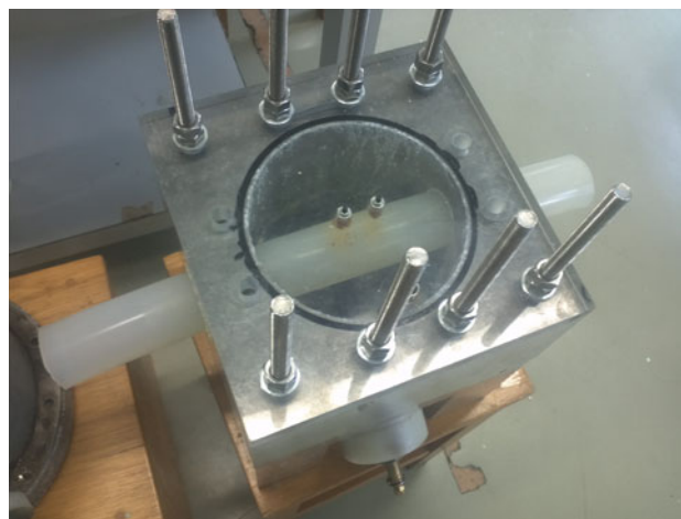
Fig. 1 View on prototype of lockable strengthened metallic vessel for continuous pressure shockwaves (50–60 MPa) with working volume of 400 mL
