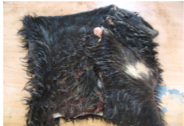
Fig. 6 The figure shows the sample of goat skin that was used for the experiment (before dehairing process)
