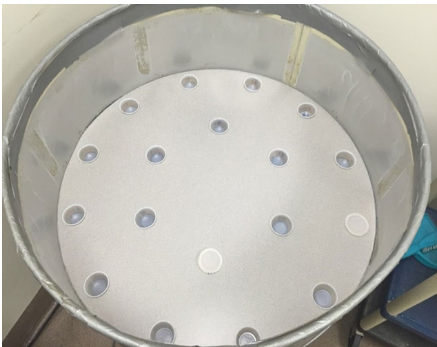
Fig. 1 Arena testing apparatus. Note In the testing arena, there are two circular arrays (rings) in which the stimuli can be placed. In the outer ring, there are 12 equidistant holes around the perimeter. Note that a cup with lid is in the 4 o'clock position. There are six equidistant holes in the center ring; there is a cup with lid in the 6 o'clock position
