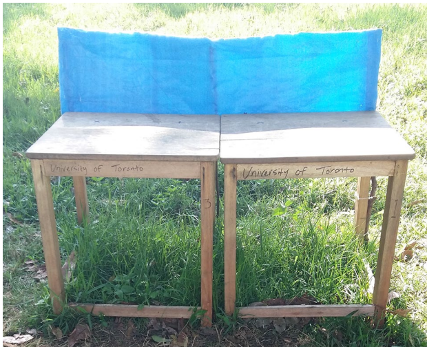
Fig. 1 The test apparatus with tarp screen attached to the back of the entire length of the platforms
