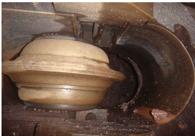
Fig. 8 Example of normal wear of a disc cutter in KrWCT project (As can be seen in the picture, there is no sign of chipping, mushrooming or irregular wear on the cutter ring, and the entire cutter ring is worn uniformly)
