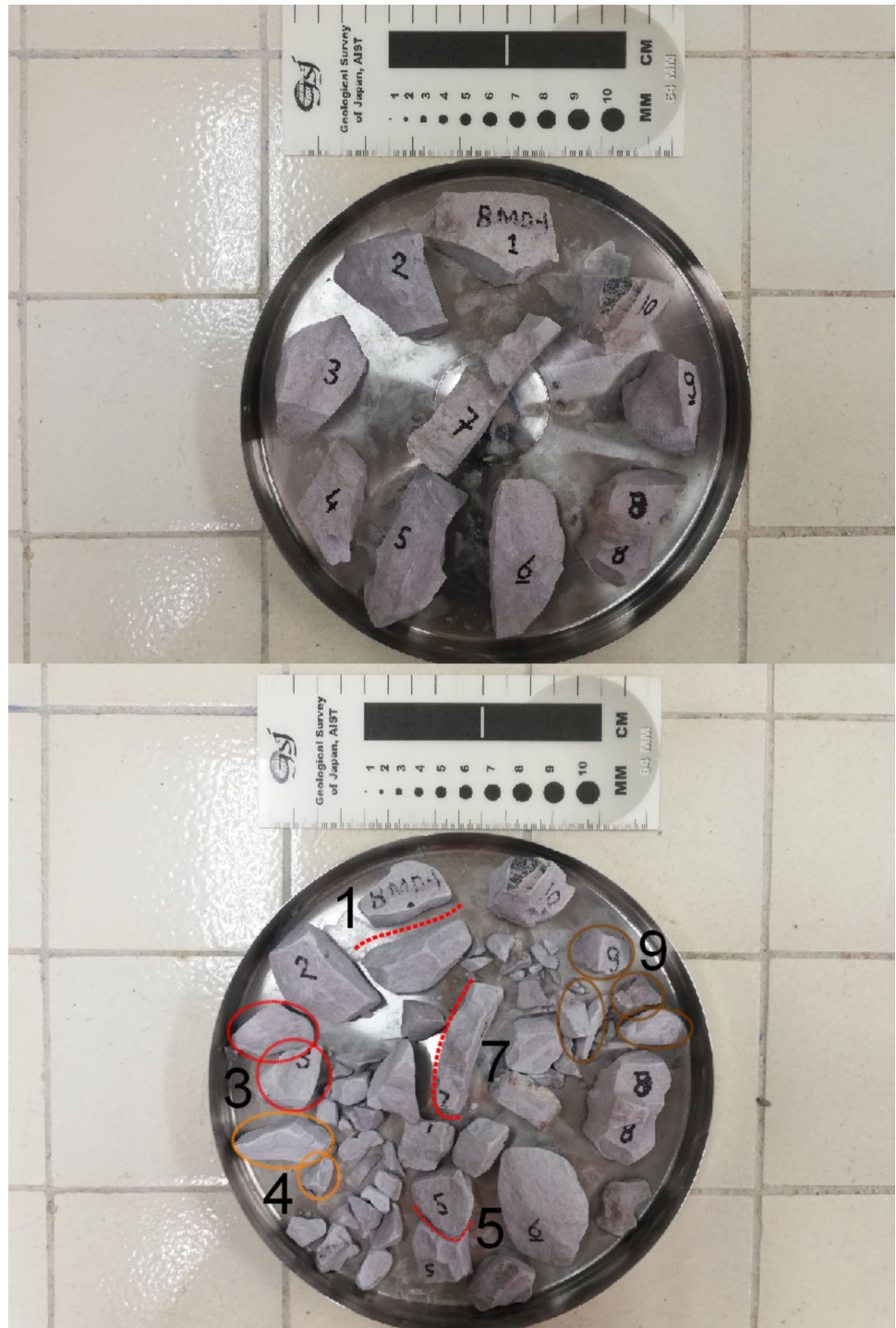
Fig. 16 Samples before (above) and after (below) two cycles of slake durability test of the case study. Lumps 1, 3, 4, 5, 7, and 9 are discarded from weighing. Lumps 3, 4, and 9 are broken into many pieces shown by dashed circles. Lumps 1, 5, and 7 are broken into either 3 or 4 pieces each having less than half of the original lump weight. Lumps 2, 6, 8, and 10 are included in the calculations since they lost less than half of the original lump by weight
