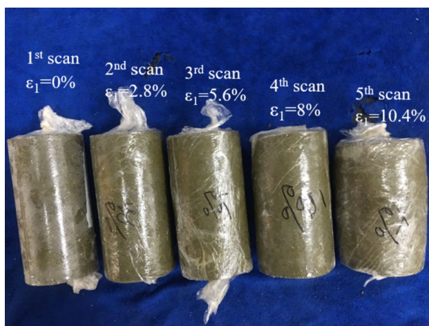
Fig. 6 Specimens after CT scanning test
