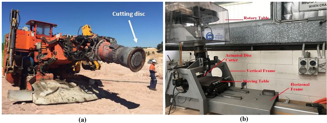
Fig. 1 Source of the data collected for this study with (a) field trials conducted for ODC using the DynaCut (b) laboratory testings conducted for ADC using Wobble (Tadic et al. 2018; Xu et al. 2021)
