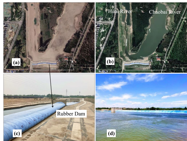
Fig. 6 The water supplied by the SNWDP-CR was used to recharge the aquifer in the Huai and Chaobai River channels in the northern part of the plain. a The remote sensing image of the rubber dam and river channel before the aquifer recharge in April 2020. b The remote sensing image of the rubber dam and river channel after the aquifer recharge in August 2020. c Rubber dam in Niulanshan. d Recharge the aquifer by using the Chaobai River channel
